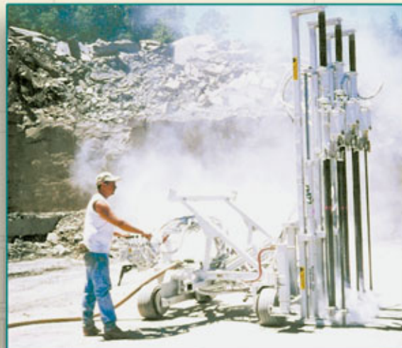
A-3 Vertical Quarry drill with a 144" drill depth.
