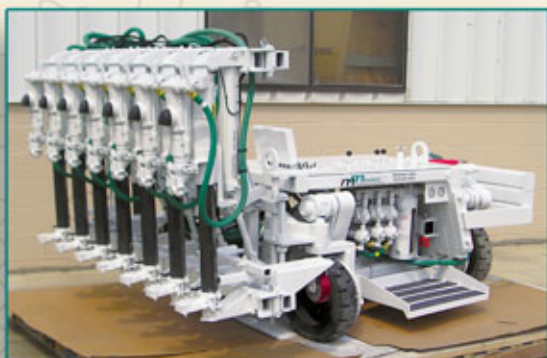
A-8SC with bed extension folded for transport.
