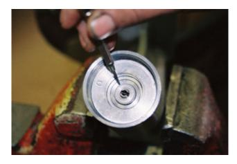
The seal can also be removed by applying a slight amount of air pressure to the return line of the vibrator. Care is to be taken not to stand in front of motor when doing this.
