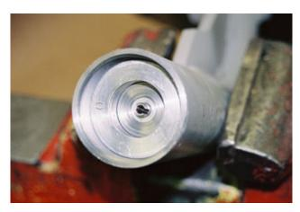
Spin the bearing on the drive shaft to check for any wear or roughness. If any roughness or wear is evident, the bearing must be replaced. Inspect the drive pin inside the motor drive shaft. If it is worn or damaged, it also must be replaced. To replace the bearing, remove the retaining ring using a pair of snap ring pliers and press bearing off shaft.
