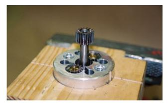
Inspect the gear cavities in the motor housing. They must be perfectly smooth. Closely check the bottom of the gear cavity. It must be perfectly flat with no sign that the drive gear is eating into the motor housing. If this is taking place, both the motor housing and drive gear must be replaced.
