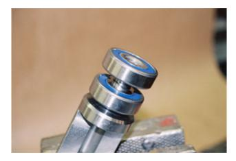
Install the bearing lock washer with its center tab in the groove and the outside tabs away from the bearing.
