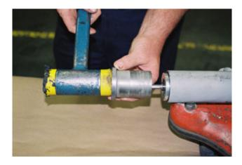
Install the sealing o-ring and seat against the motor.
