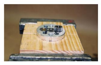
Take end cap and place small amounts of grease at three or four spots around the o-ring groove to keep o-ring in place while assembling end cap to motor housing. Install new o-ring into the groove of the end cap (old o-ring may not assure as good a seal).
