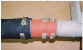
If oil is present inside the cover hose, connect the vibrator to a 4 g.p.m. test stand or vibrator circuit on a machine and run vibrator to check for oil leaks at the hose connections or the hoses themselves. If no leaks are apparent, disconnect the extension hoses from the motor hoses. If vibrator is equipped with a sensor for a MINNICH Auto Vibe system, unplug the extension cord at this time also.
