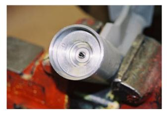
Remove the seal from the motor housing using a hooked tool.
