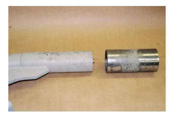
Pull motor with attached hoses (and cord from Auto Vibe sensor, if present) from motor tube.
