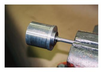
Remove seal washer and seal from motor housing. Check seal washer to be certain it is perfectly flat and not bowed due to pressure.
