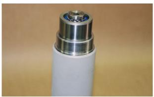
Apply #1 Permatex or equivalent thread sealer to the threads of the eccentric housing and screw into motor housing. Place a pipe wrench on tip of the eccentric housing and tighten it securely. Test the vibrator on a 4 g.p.m. test stand or using a vibrator circuit on a machine.
