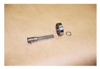
To replace the drive pin, the bearing must be removed as described above. Push the drive pin from the drive shaft. Install the new pin until the ends of the pin are flush with the edges of the shaft.
