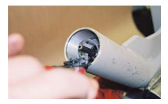
Clamp motor drive shaft with a pair of vice grips. Tap the vice grips with a mallet until the shaft and bearing assembly comes out.
