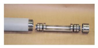
Clamp the eccentric assembly in a vise in a vertical position. Using a hammer and screwdriver, straighten the tab on the locking washer that is engaged into the notch of the bearing lock nut.
