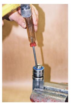
Using a spanner wrench, remove the nut from the eccentric weight by turning it counterclockwise.
