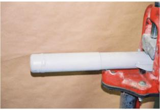
Place a pipe wrench on the extreme tip of the of the eccentric housing and remove it by turning it counterclockwise.
