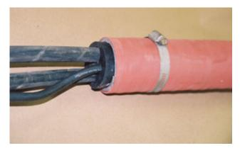
Cut the clamp band from the protective hose with a cutting wheel or a hammer and sharp chisel. Slide the protective hose back, revealing the two clamp bands securing the cover hose to the motor housing. Cut these two clamps also as above. If protective hose has to be cut to be removed, do so with care so as not to damage the cover hose.
