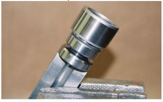
Make sure that the inside of the eccentric tube is clean before starting to install the eccentric weight assembly into it. Insert the eccentric assembly into the housing with the bearing housing towards the open end. Using a rubber mallet, tap the assembly into the tube until the bearing housing is flush with the end of the eccentric tube.
