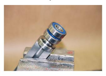
Clean off the bearings with solvent or diesel fuel. Spin the bearings to check for roughness or wear. If roughness or wear is detected, the bearings must be replaced. It is recommended that new bearings and shims be installed when rebuilding an eccentric assembly. It has been determined that relubricated bearings do not last as long as new bearings.
