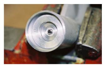
Insert the drive shaft and bearing assembly into the motor housing. Using a piece of tubing or a socket matching the outside diameter of the outer bearing race, carefully tap the assembly into the housing. Tap on the bearing until the slot for the locking ring is exposed. Install the retaining ring using a pair of snap ring pliers.
