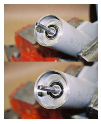
Install the sealing o-ring into the motor housing flush against the motor. The reason for this o-ring seal is to keep any liquids from getting past the motor in either direction. In case of a motor seal failure it will keep the oil from getting past the motor into the upper part of the vibrator assembly.
