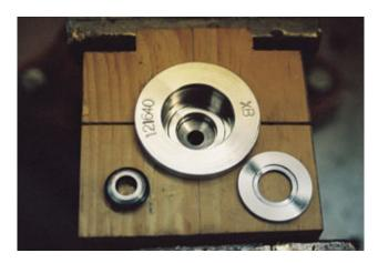
An easy way of doing this is to put washer face down (side with recess) on a flat surface and put down-pressure with two fingers on opposite sides of the rim and see if it sits firmly or wobbles. If washer is not flat, replace it. Wash all parts in clean solvent or diesel fuel.
