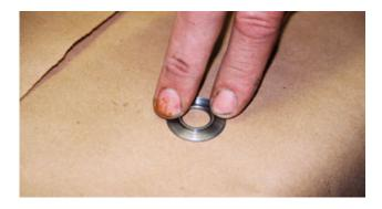
If washer is not flat, replace it. Install seal washer with machined step towards the seal assembly.
