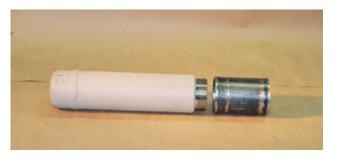
After the eccentric assembly is removed from the housing, remove the bearing housing from the bearings on one end of the eccentric assembly.
