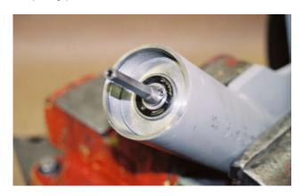
Turn motor housing over in the vise (gear pockets facing up). Dip the motor drive gear and shaft in clean hydraulic oil and install it in the housing while rotating the drive shaft to ensure proper engagement of gear and drive pin in drive shaft.
