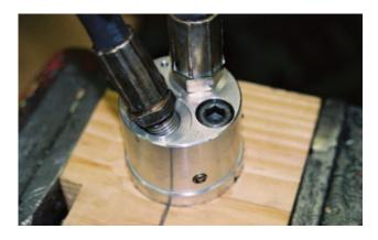
If motor was equipped with a sensor for the MINNICH Auto Vibe system carefully install the sensor at this time. Install stand-off-s between the sensor and motor end cap. Use new socket head cap screws to secure the sensor. If using old cap screws apply Loctite 242 (blue) before installing screws. Make sure that one flat washer is placed between the sensor and head of each screw. With a 3/32" (.093") allen wrench tighten to 12 in. lb. torque. Secure the cable to a motor hose with tie warps.
