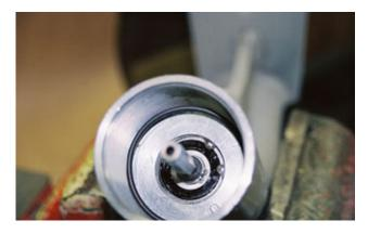
Install the motor lock nut and tighten securely with motor lock nut spanner wrench.
