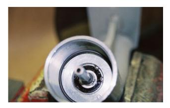
Install the motor lock nut and tighten securely using the motor lock nut spanner wrench.
