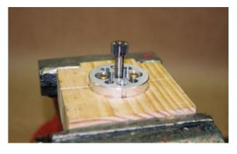
Dip the two idler gears in clean hydraulic oil and install them in pockets on either side of the drive gear. Rotate the output shaft to insure that the gears turn freely.
