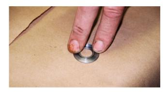
Spin bearing on the drive shaft to check for any wear or roughness. If any wear or roughness is evident, the bearing must be replaced. Inspect the drive pin inside the motor drive shaft. If it is worn or damaged, it also must be replaced. To replace the bearing, remove the retaining ring using a pair of snap ring pliers and press the bearing off the shaft.
