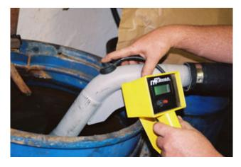
The assembled vibrator should be tested for the maximum starting pressure required to operate the vibrator which is a maximum pressure of 200 psi.
