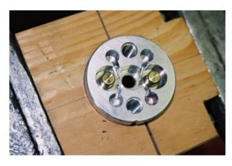
Remove motor housing from vise and using a pair of internal snap-ring pliers remove the large retaining ring securing the drive shaft assembly. Clamp the motor drive shaft in a vise horizontally. The shaft is hardened and the vise will not mar it. Tap the motor housing with a rubber mallet while rotating it until the bearing assembly comes out.
