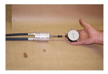
If a complete vibrator assembly is to be tested, it should be suspended in a container of water to cool the bearings in the eccentric tip assembly. Connect the vibrator assembly to a 4 g.p.m. hydraulic test stand or to a vibrator circuit on a machine.
