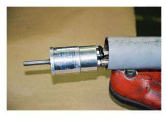
Tap with a rubber mallet, if necessary, on the motor drive tube to seat the motor into the housing.
