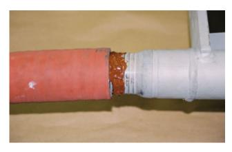
Install two band type hose clamps over the cover hose over the barbs and secure cover hose to motor tube following directions provided with clamp tool. Use only PunchLok type hose clamps in this position - screw type hose clamps interfere with the installation of the protective hose.
