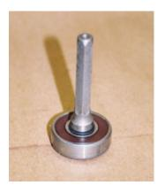
If bearings are to be repacked, carefully remove the seals from the bearing and wash out with clean solvent and dry. Repack bearing to 50% fill with high speed, high temperature, non-water soluble grease (Polyrex EM2 or equal). Carefully reinstall the seals and work grease into bearing by rolling it back and forth before installing it on the drive shaft.
