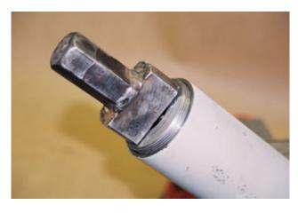
Finish vibrator assembly by installing the eccentric assembly as described in Section I.
