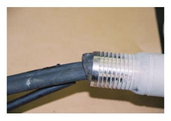
Remove the eccentric housing assembly from the motor tube as described in section I. Remove the motor lock nut with motor lock nut spanner wrench. Also remove sealing o-ring from motor housing. Remove motor housing from fixture or vise. Slide motor tube into motor bump tube. Strike open end of bump tube and motor housing assembly sharply on a hard surface (floor or metal plate) until the motor slips free from the motor housing.
