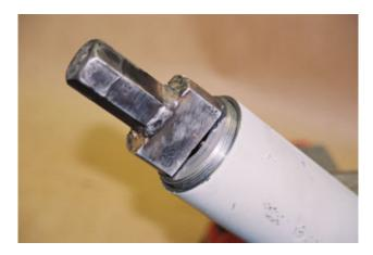
It is recommended that the vibrator be connected to a 4 g.p.m. hydraulic test stand or a vibrator circuit on a machine to be tested for seal leakage and correct rotation. The motor shaft should rotate counterclockwise when looking at the end of the shaft.
