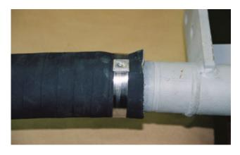
Install upper hose plug over the two hoses (and cable) and slide it into the cover hose until it is flush with the end. Secure tightly with a screw type hose clamp.
