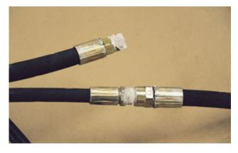
Apply #1 Permatex or equivalent sealer on the barbed end of the motor housing. Slide cover hose over the extension hoses (and cable) and completely over the barbs on the motor housing.
