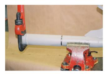
Slip the threaded end of the eccentric housing assembly into the bump tube. Strike the open end of the bump tube and eccentric assembly sharply on a hard surface (floor or metal plate) until the eccentric assembly slips free from the housing.
