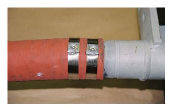
Slide protective hose over the cover hose until it is over the motor housing. Secure it in place with a single band type hose clamp. The protective hose is installed in a high wear area to protect the cover hose and attaching clamps.
