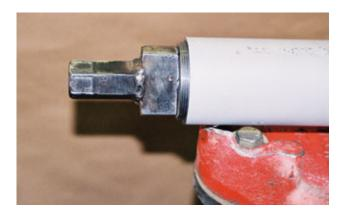
With a pair of internal snap ring piers remove large bearing retaining ring from motor.
