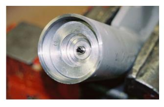
Before reassembling motor, check machined seal washer to be certain that it is perfectly flat and not bowed due to pressure. An easy way of doing this is to put seal washer face down (side with recess) on a hard , flat surface and put down-pressure with two fingers on opposite sides of rim and see if it sits firmly or wobbles
