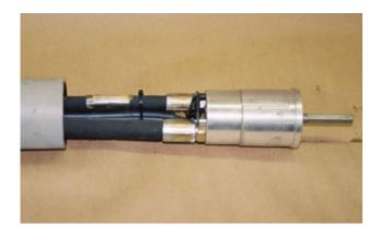
Place motor housing in vise with the hoses up (either a fixture or with vise jaws gripping motor housing on the grooves). If motor is equipped with a MINNICH Auto Vibe sensor, using a 3/32" (.093") allen wrench, carefully remove the two socket head capscrews securing sensor to end cap. Cut the tiewraps attaching cord to motor hose. Remove sensor and then both motor hoses.
