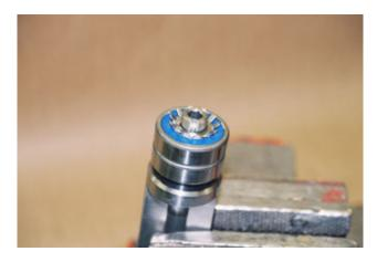
Install the bearing locknut with the chamfer toward the bearing. Tighten the nut securely and bend one of the lock washer tabs into one of the slots in the side of the nut.
