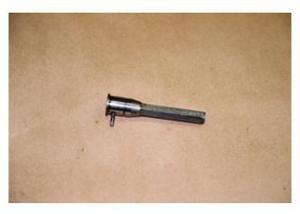
It is recommended that a new bearing be installed when rebuilding the drive shaft. It has been determined that relubricated bearings do not last as long as new bearings. Install the bearing by pressing it onto the shaft. Install the retaining ring to secure the bearing in place.
