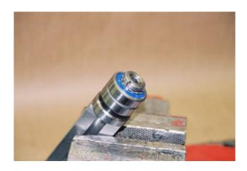
Repeat this process with the bearings on the other end of the eccentric weight. Inspect bearing housing for any signs of a bearing having a loose fit and having spun in the housing. Replace housing if it shows any signs of the bearing having spun. Install bearing housing over bearings on one end of the eccentric assembly
