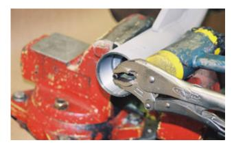
The shaft is hardened and the vice grips will not mar it. Remove the seal washer exposing the seal housing.
