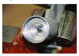
Since it is difficult to tell whether it is the internal shaft seal o-ring or the outer o-ring that is bad replace both using a new seal assembly. Dip seal assembly in oil and install it with the chamfered side of the seal housing towards the motor. Push it firmly into place, taking care that the external o-ring is properly seated.
