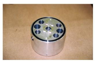
Install the motor end cap and secure with two allen head cap screws. Dip cap screw threads in clean hydraulic oil before inserting them in motor housing. Tighten them evenly to 20 ft. lb. of torque with a 5/16" (.312") allen wrench. Turn output shaft to insure that the motor will turn freely.
