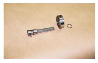
To replace the drive pin, the bearing must be removed as described above. Push the drive pin from the drive shaft. Install new pin until the ends of the pin are flush with the edges of the shaft.
