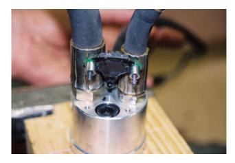
Place vibrator motor housing back in the vise. Slide the motor hoses into the motor housing. Align the grooves in the sides of the motor with the locating balls in the motor housing and slide the motor into place.
