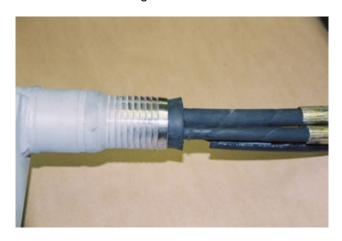
Apply thread sealer on hose end fittings and connect the extension hoses. Connect extension hose marked with AP@ to the vibrator motor hose marked with AP@ (pressure hose). Connect other extension (return) hose and tighten both securely. Connect Auto Vibe extension cable at this time if applicable.
