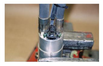
Using a 5/16" (.312") allen wrench remove the two socket head capscrews from the end cap and remove end cap and sealing o-ring. Inspect end cap for signs of gears digging in. Replace if necessary. A slight burnished pattern from the gears is common.
