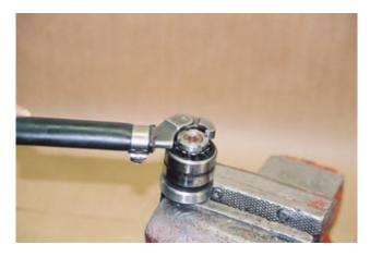
Remove the two bearings and shims from the eccentric weight. Repeat the procedure on the other end of the eccentric weight.
