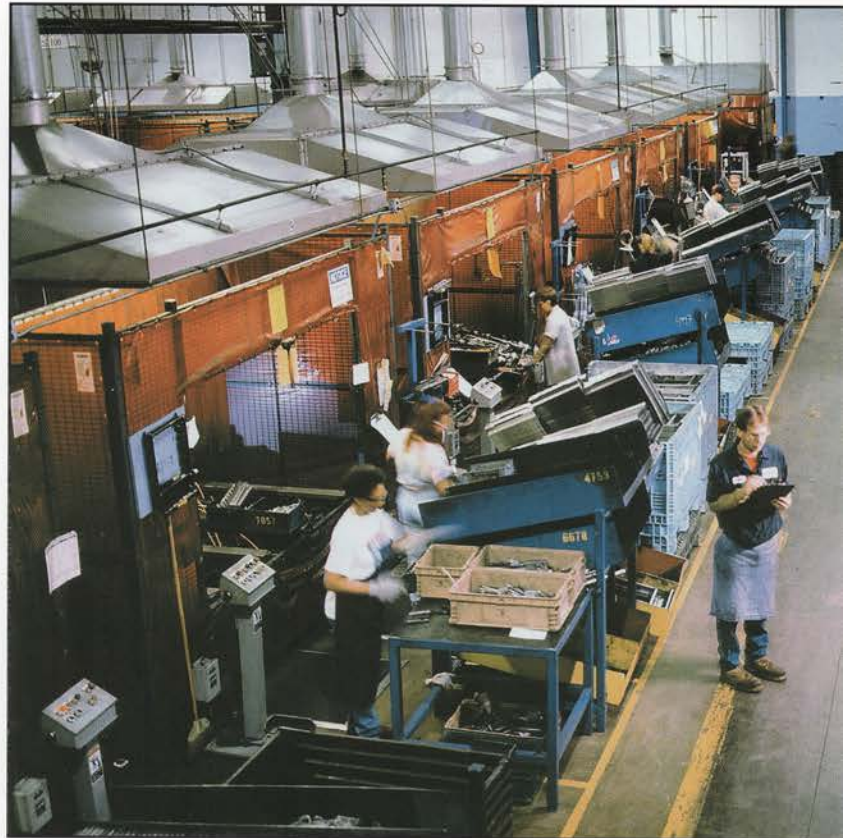
Assembly operations are organized as sequential welding cells. The arrangement is conducive to the use of common equipment while meeting the specific needs of each application.
