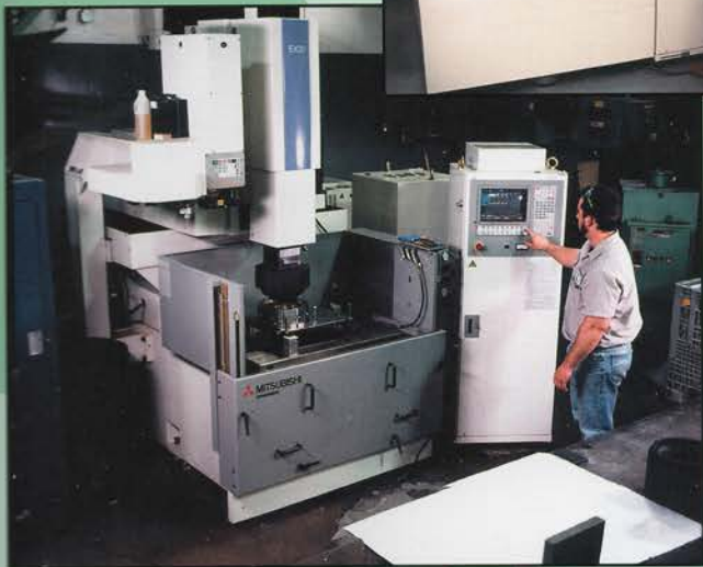
A Mitsubishi EX30 Diesinking EDM and a Mitsubishi FX20 Wire EDM guided by digital engineering systems allow for the generation and reproduction of complex precision tooling
