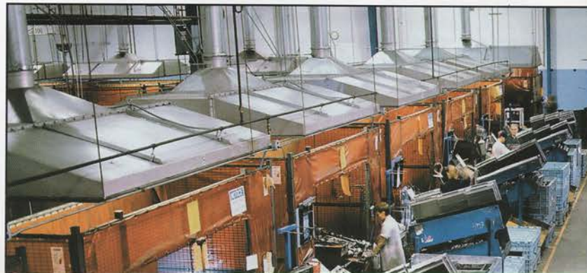
This computer controlled tube bending and forming cell involves four transfer stations, a bender with two plane capability and final trim press.
