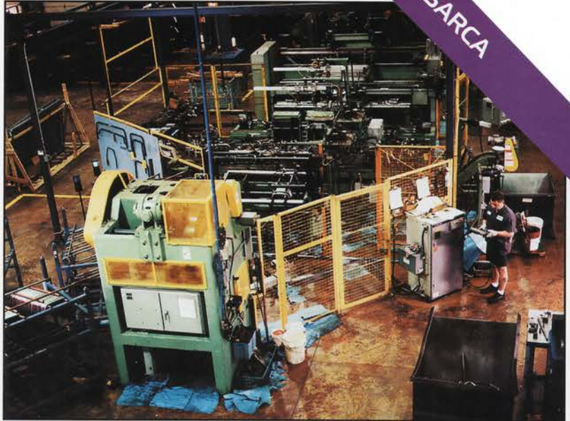
This computer controlled tube bending and forming cell involves four transfer stations, a bender with two plane capability and final trim press.
