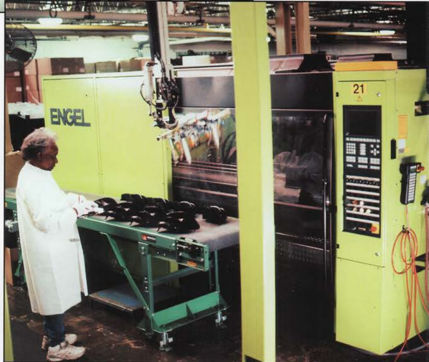
This Engle injection molder features closed loop microcomputer process controls and robotic removal and trimming. The sophisticated control system allows for maximum productivity with internal monitoring of all critical functions.
