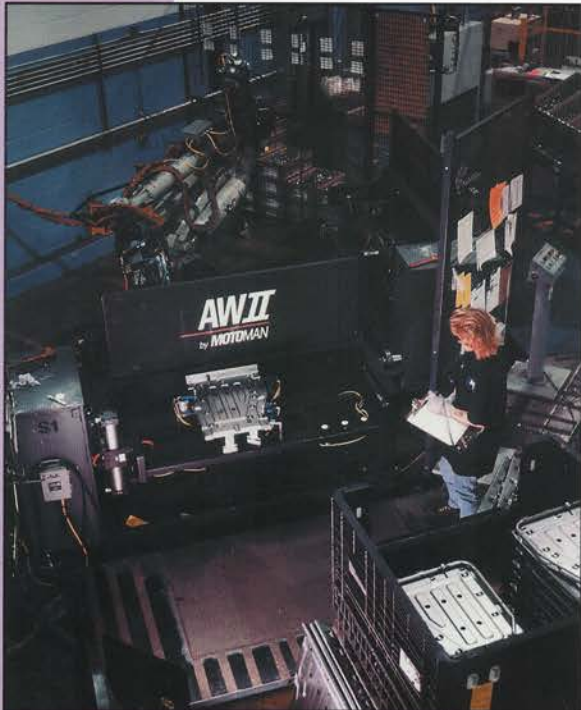
Computer monitoring of robotic welds produces a specific assembly in an accurate, repetitive and efficient manner.
